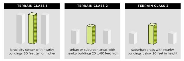
Figure 5: Terrain classes are based on a building's potential for wind exposure.<sup>15</sup>
