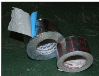
Figure 7. Two UL rated duct tapes (Butyl tape, left roll, and Aluminum foil tape, right roll).
