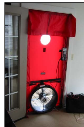
Figure 22. Blower door being used to pressurize home.
