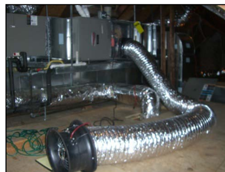
Figure 21. Duct leakage testing
