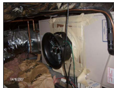
Figure 20. Airflow testing using a duct blower.
