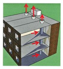
damper that balances unit flows. Additional small, individual fans with relatively low flow are efficient and quiet.
